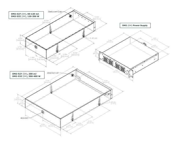
Photonics Industries DM Dual Head Series nanosecond lasers have a separate external power supply box, no longer requiring an external controller or utility module. The RF driver is located in the laser head, and all control electronics and connections for operation and control of the laser can be found on the back panel of the compact laser head.
