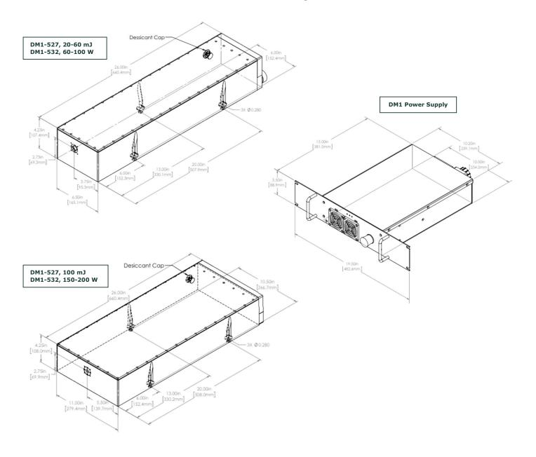
Photonics Industries DM Series nanosecond lasers have a separate external power supply box, no longer requiring an external controller or utility module. The RF driver is located in the laser head, and all control electronics and connections for operation and control of the laser can be found on the back panel of the compact laser head.
